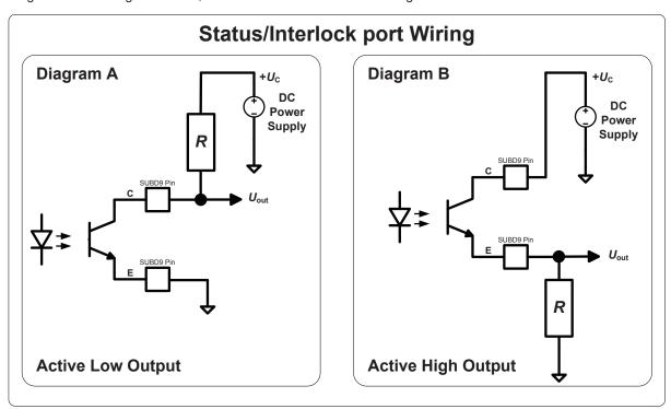
In the Diagram A Active Low Output, the output signal  $U_{\rm out}$  switches to GND when the corresponding LED is ON. In the Diagram B Active High Output, the output signal  $U_{\rm out}$  switches to  $+U_{\rm C}$  when the corresponding LED is ON. When the output signal  $U_{\rm out}$  is switched to GND, its value is lower than 0.2 V. When the output signal  $U_{\rm out}$  is switched to  $+U_{\rm C}$ , its value is equal to  $+U_{\rm C}$ .
